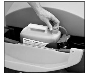
Attach the cap to bottle and detergent is automatically diluted to the proper ratio.
